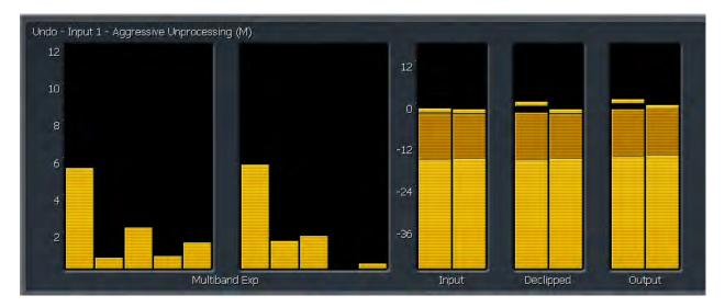
"blips") for the input audio, audio after the declipper, and after the multiband expanders (Output).
