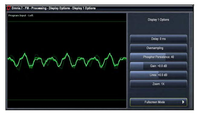
When the oscilloscope is selected as the current type of instrumentation, controls for adjusting its display
