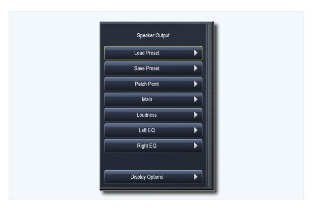
• Note: Keep in mind that although some of the features, terms, and tools in the Monitor Output sections are similar or identical to their counterparts in Omnia.7's various processing cores - such as the term "preset" - they have no impact on the air. Monitor Outputs only control what you hear through the Speaker or Headphone outputs.
