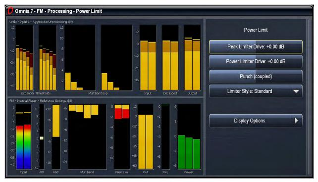
Controls for adjusting the Power Limiter are found in the FM> Processing> Power Limit menu.
