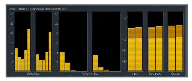
• The **Expander Ratio** meters indicate the current ratio of expansion relative to the detected incoming dynamics. Less dynamic source material will have a higher expander ratio compared to content that is more dynamic.
