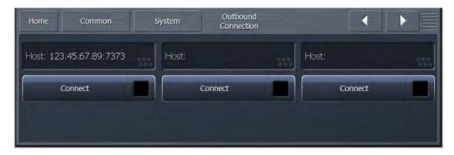
One example of how this can be used is for technical support. By creating an outbound connection, you are connecting to the support engineer's NfRemote computer which in turn allows them to control your Omnia.7.
