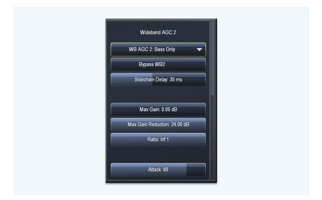
Omnia.7 allows you to insert an additional (and rather versatile) AGC into the processing chain after the
