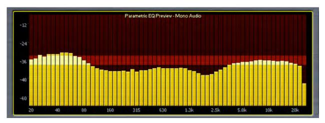
You will now be able to see the curve of the PEQ in the RTA display window. You can also view the curves of each band of the multiband compressor by selecting one of the Solo band buttons. Since the Solo bands relate to a dynamic section of the processing core, lowering the Averages slider will yield more of a "real time" view.
