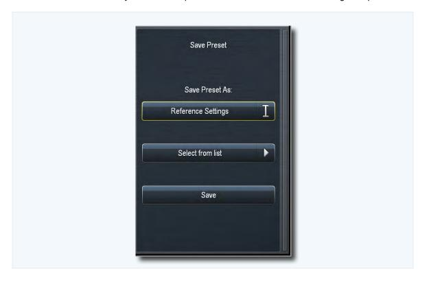
The current preset, regardless of whether or not it has been modified, can be renamed by highlighting and selecting the **Save Preset As** control which will bring up the on-screen keyboard. Rotating the controller clockwise and counter-clockwise provides navigation through the keyboard; moving it to the right selects the highlighted character. Select "OK" and then **Save** to save the preset with the new name.
