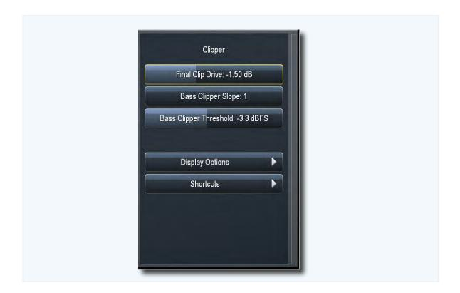
The Final Clip Drive control sets the drive of the final clipper. Decreasing the drive (moving the slider to the left) reduces the amount of clipping. Conversely, increasing the drive (moving the slider to the right)
