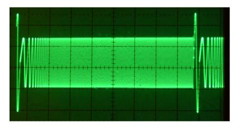
this is the shape you would see if your STL or exciter had a flat high frequency response: Any deviation from a flat high frequency response means a loss of loudness and/or stereo separation.
