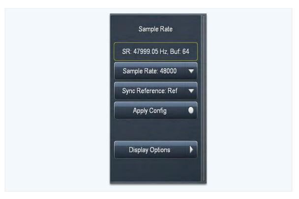
The main AES XLR inputs can accept audio with a reference of either 44.1kHz (for HD Radio) or 48kHz (for DAB). To set the sample rate, navigate to the **System > System Configuration > Sample Rate** menu and set the unit's sample rate to match that of the incoming signal and the **Sync Reference** control to "Main Input".
