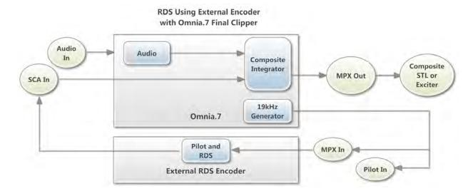
Be sure to enable the proper MPX input for RDS use (Input 1 or Input 2) in the RDS Mode menu, and set the MPX 2 Output control to the 19kHz Generator mode. The MPX 2 Output control can be found in the RDS Menu, the FM Processing Output menu, and in the main I/O menu.
