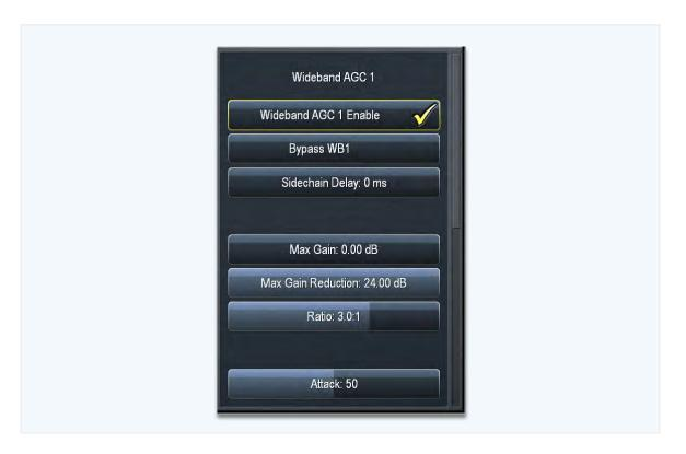
reduction, ratio, attack, release, progressive release, target, gate threshold, and freeze threshold controls.
