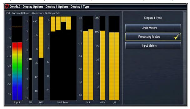
• The **Input Meters** menu allows you to monitor the audio levels entering Omnia.7 with ITU-R BS.1770 bargraph meters.
