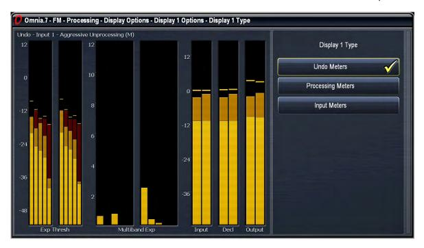
• The **Processing Meters** menu allows you to display the levels and activity of Omnia.7's various gain stages and processing sections. A complete explanation of these meters is provided in Chapter 5.
