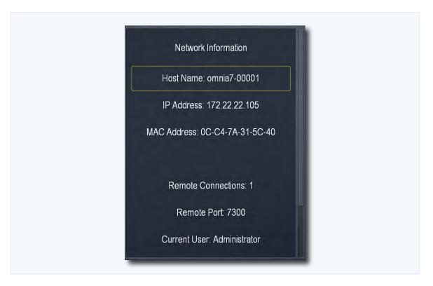
MAC address of the unit. It also indicates how many users are remotely connected, the remote port number, and the security level of the current user.
