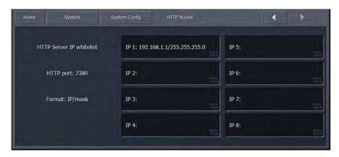
Using a web browser of your choice (and the actual IP address of your Omnia.7 to replace the sample address here), enter "<a href="http://192.168.1.1:7380">http://192.168.1.1:7380</a>". This will bring up the HTTP server home page which contains a link to the NfRemote software. Download, locate and install the software. Once installed, assign a "friendly" name of your choice in the "Comment" field, enter the IP address and password, and click "Connect".
