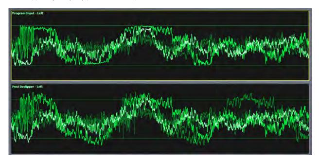
The second stage of Undo is a multi-band expander that is designed to restore dynamic range to audio that has been excessively compressed.
