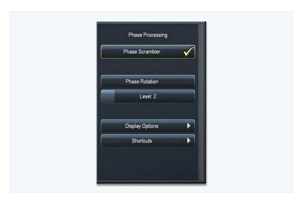
that the amount of phase rotation is now adjustable by using the **Level** control.
