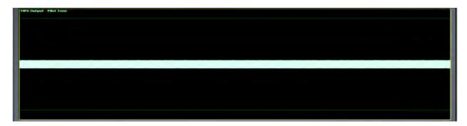
Note that what you are seeing here is the actual pilot extracted from the entire MPX signal. To see just how tightly the composite signal is packed, compare the complete MPX signal to one with no pilot and note that the peak level actually increases when the pilot is removed! This is exactly the opposite of what you will observe with any other processor (except for Omnia.9).
