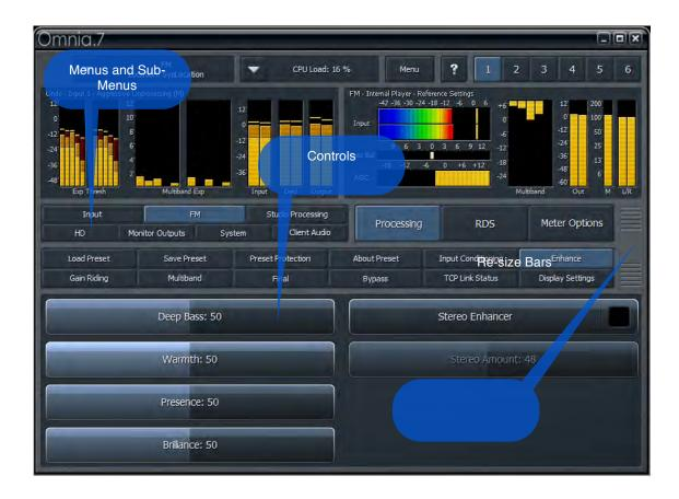
The screen in this view is divided into three sections; the top shows the displays, the middle shows the menus and sub-menus, and the bottom contains the controls.
