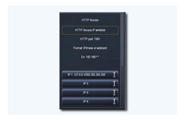
• Enter the IP address and subnet mask information using the following example as a guide: 192.168.1.0/255.255.255.0 (The beginning of the IP range followed by the subnet mask, separated by a forward slash). Standard TCP/IP wildcards such as the asterisk (" \* ") are also supported. Up to eight addresses can be stored.
