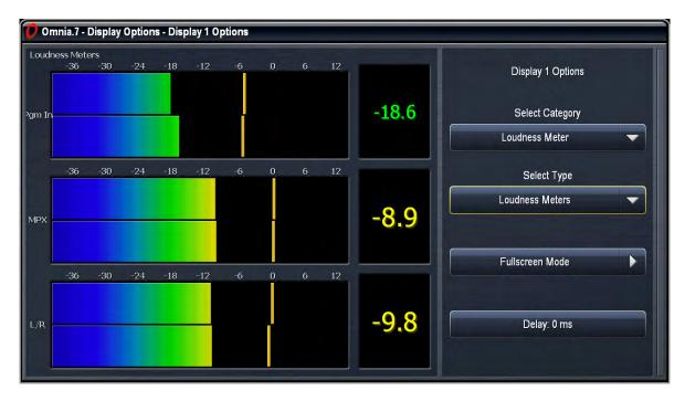
Selecting the Short Term Loudness Graph provides a graphical representation of loudness over time. Because it does take addition CPU resources to create the graphs, graphic is turned "off" by default and must be enabled for each processing core (FM and HD) in the Meter Options > Meter
